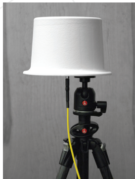
Tripod-mountable with ¼-20 PEM on top plate, shown below.
